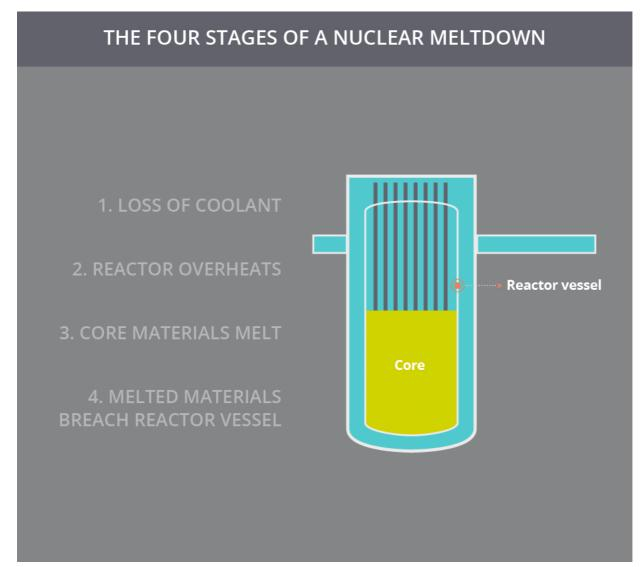
When all safety systems fail, loss of coolant in a reactor will quickly build up heat and melt the radioactive materials.
