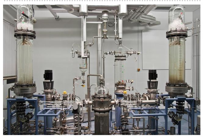
A glass scale model of a nuclear power plant in Essen, Germany, will help scientists test ways to reduce the risk of meltdowns. Image courtesy of sCO2-HeRo
