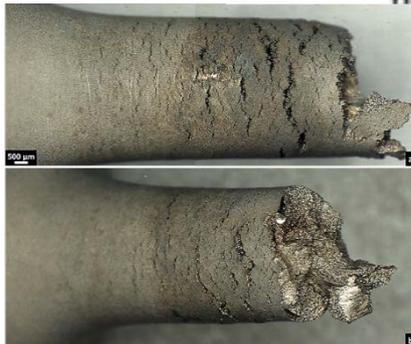
GH3535 creep rupture test (190 MPa, 700°C)
