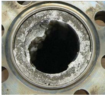
FIGURE 9. Salt solidification in the inside a pipe of a FLiNaK experiment.
