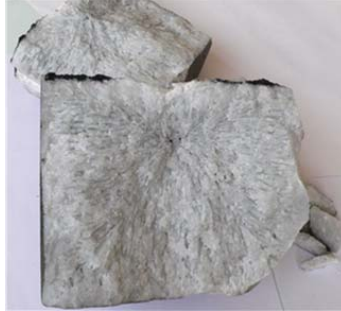
FIGURE 8. Complex structure of a solidified LiF-NaF-KF eutectic (FLiNaK).
