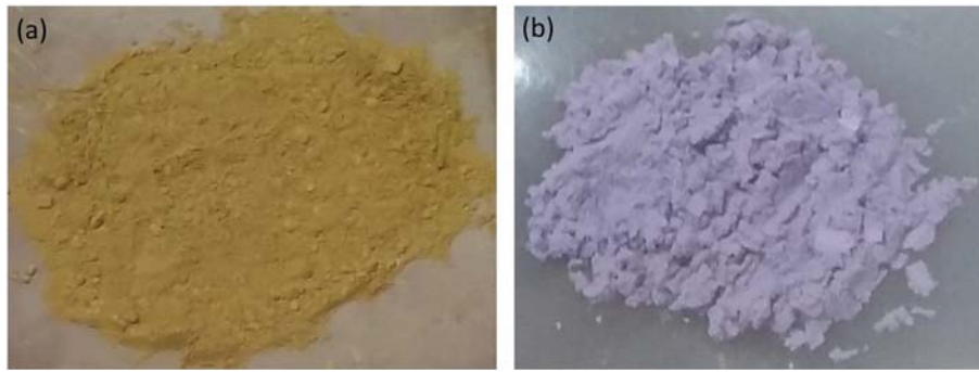
Fig. 1. Photos of the initial material PuO 2 (a) and final product PuF 3 (b). For the colour photos, please refer to the Web version of this article.
