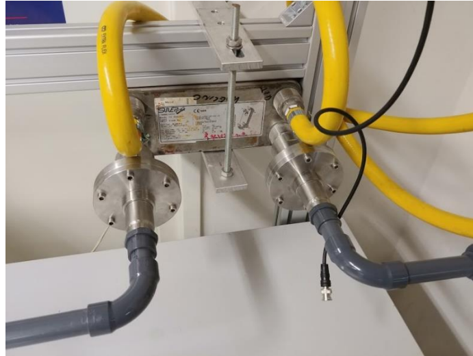
Figure B.3: Heat exchanger coupled with the loop and 2 tubes which contain the cooling water
