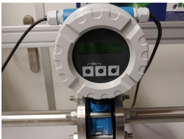
Figure B.2: The flowmeter that kept track of the liquid flow rate. The meter was linked to the computer and used a special made software. The rates on the meter itself are given in \text{dm}^3/\text{min} and on the computer in \text{L/s} .
