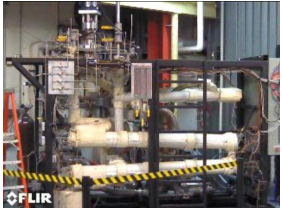
Forced Flow FLiBe Loop Thermal Image, Operating 2GPM, 700°C Hot Side, 650°C Cold Side University of Wisconsin - Madison
